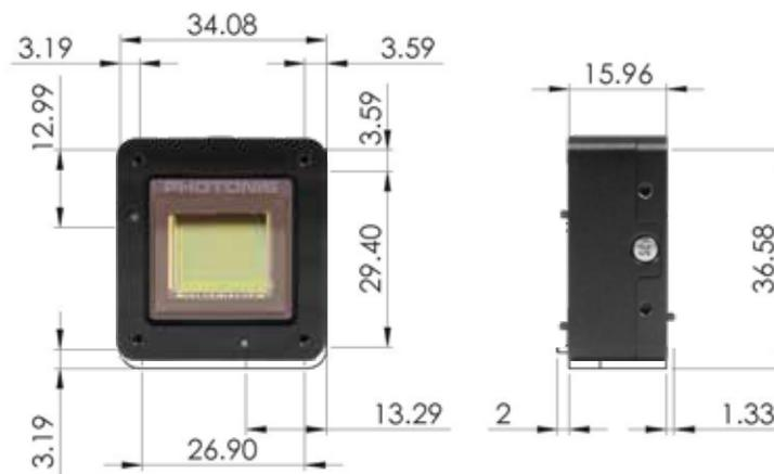
NOCTURN XS Camera is powered by the LYNX CMOS or KAMELEON Color imaging sensor, optimized for low light level imaging.
